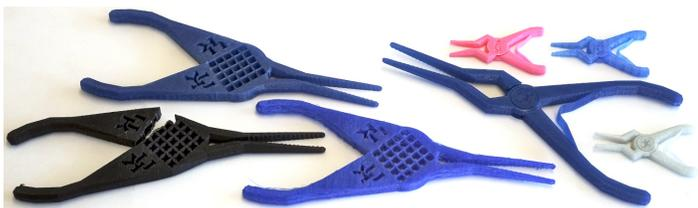
**Macro Metamaterials.** A metamaterial is an object in which different properties are obtained not by use of different materials or multiple-part assemblies, but solely by engineering the shape of the structure. The concept of using a single homogeneous material is particularly attractive for 3D printing, but conventional repeated-cell structures (left) don't deliver the desired mechanical properties. Our 3D-printed macro-scale metamaterial structures (right) operate smoothly without degrading.
