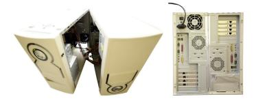
**HAK – Half-powered Athlon cluster in Kentucky.** We have long known that the power supplies in most of our nodes are running at only about 1/3 their design output. We also have found that power supplies are the most commonly failing components. In June 2010, we built HAK to answer the age-old question of whether nodes sharing commodity power supplies is beneficial.
