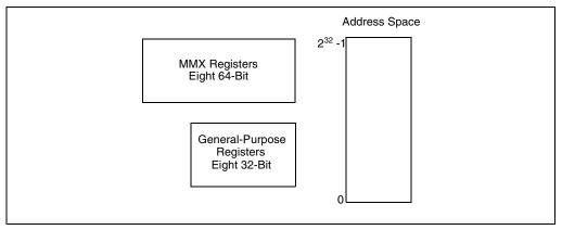
Figure 9-1. MMX Technology Execution Environment
