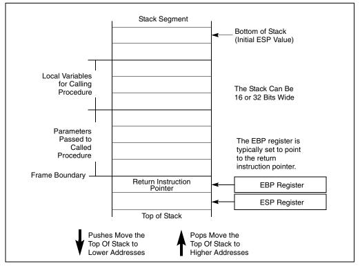
Figure 6-1. Stack Structure
