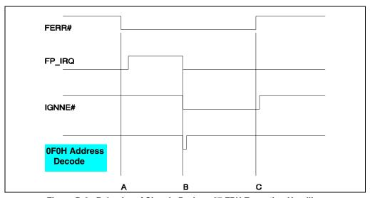
Figure D-2. Behavior of Signals During x87 FPU Exception Handling
