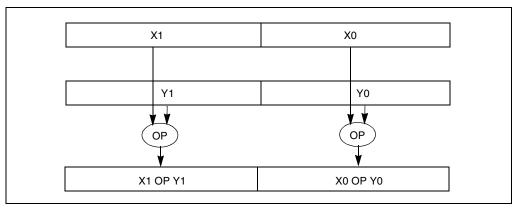
Figure 11-3. Packed Double-Precision Floating-Point Operations
