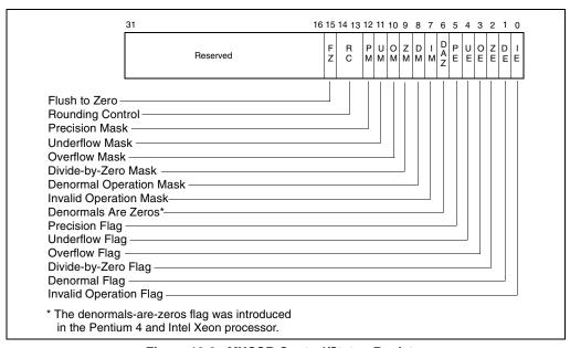
Figure 10-3. MXCSR Control/Status Register
