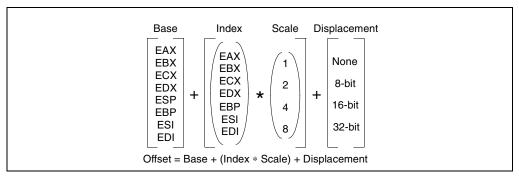
Figure 3-9. Offset (or Effective Address) Computation
