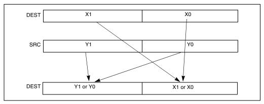
Figure 11-5. SHUFPD Instruction Packed Shuffle Operation
