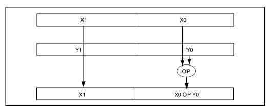
Figure 11-4. Scalar Double-Precision Floating-Point Operations
