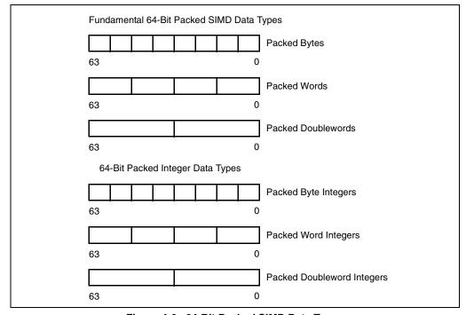
Figure 4-6. 64-Bit Packed SIMD Data Types
