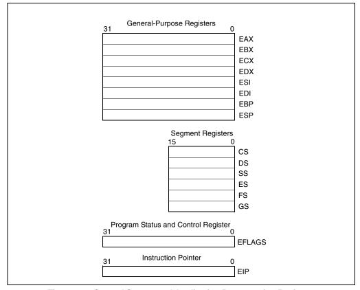
Figure 3-3. General System and Application Programming Registers
