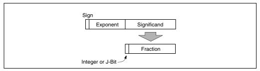
Figure 4-10. Binary Floating-Point Format
