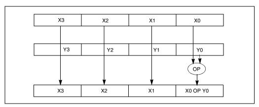
Figure 10-6. Scalar Single-Precision Floating-Point Operation
