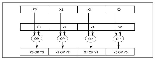
Figure 10-5. Packed Single-Precision Floating-Point Operation
