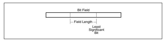
Figure 4-5. Bit Field Data Type
