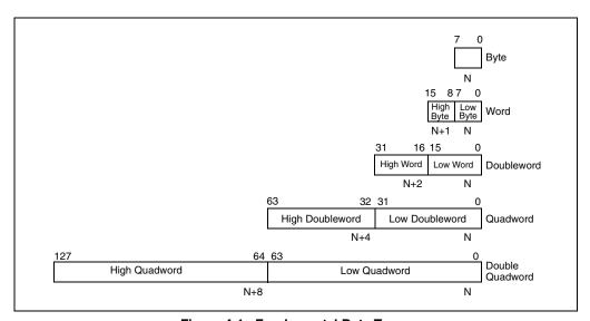
Figure 4-1. Fundamental Data Types
