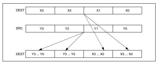
Figure 10-7. SHUFPS Instruction Packed Shuffle Operation
