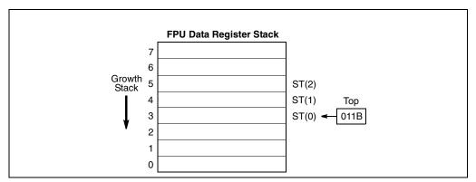
Figure 8-2. x87 FPU Data Register Stack
