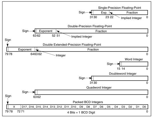
Figure 8-13. x87 FPU Data Type Formats
