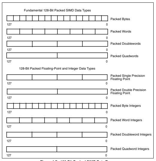
Figure 4-7. 128-Bit Packed SIMD Data Types
