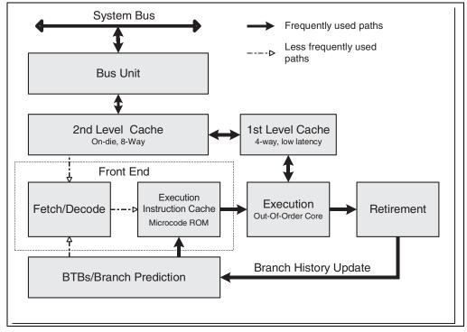
Figure 2-1. The P6 Processor Micro-Architecture with Advanced Transfer
