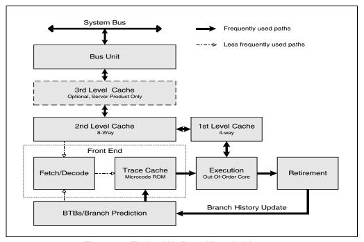
Figure 2-2. The Intel NetBurst Micro-Architecture
