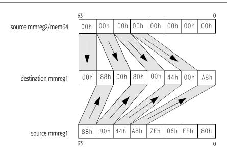
In the functional illustration of the PUNPCKHBW instruction, the 8-bit values from mmreg1 are stored in the low-order 8 bits of the 16-bit result. The mmreg2/mem64 source operand is set to all zero bits so it can provide zero fill in the high-order 8 bits of the 16-bit result. This is a method that can be used to expand unsigned 8-bit values into unsigned 16-bit operands for subsequent processing that requires higher precision.
