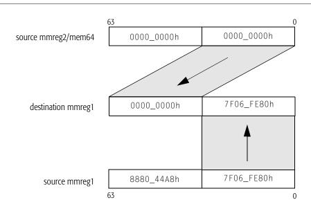
In the functional illustration of the PUNPCKLDQ instruction, the 32-bit value from mmreg1 is stored in the low-order 32 bits of the 64-bit result. The mmreg2/mem64 source operand is set to all zero bits so it can provide zero fill in the high-order 32 bits of the 64-bit result. This is a method that can be used to expand unsigned 32-bit values into unsigned 64-bit operands for subsequent processing that requires higher precision.
