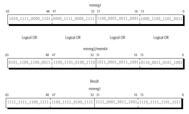
In the functional illustration of the POR instruction, the 64-bit source value is logically OR'd to the 64-bit destination value, and the result is stored in the destination register.
