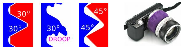
A 45° angle is printable by nearly all printers, but the choice of angle is printer-dependent and even more precise threads can be obtained by accounting droop.
