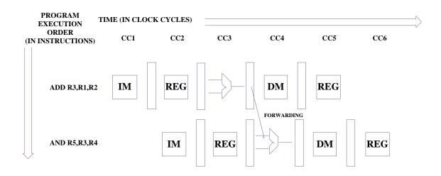
Figure 21: Forwarding the pipeline saves the cost of a stall cycle
