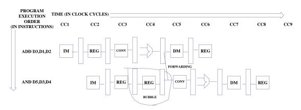
Figure 24: Clock cycle 4 repeats the operations done during clock cycle 3 to introduce a pipeline bubble.
