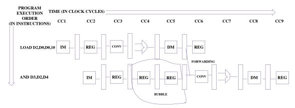
Figure 23: For same problem the hazard forces the AND instruction to repeat in the clock cycles 4 and 5 what it did in clock cycle 3.
