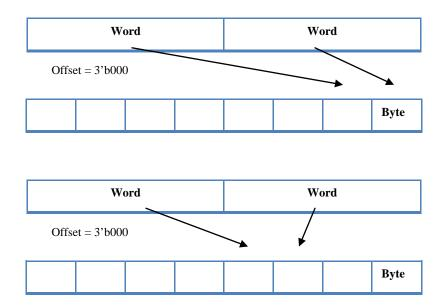
Figure 17: Type conversion- saturation arithmetic rules for packing data
