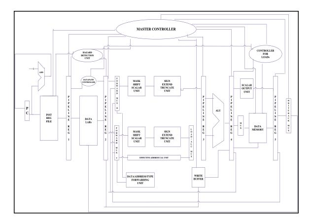
Figure 20: Block diagram of DATA LARs architecture design
