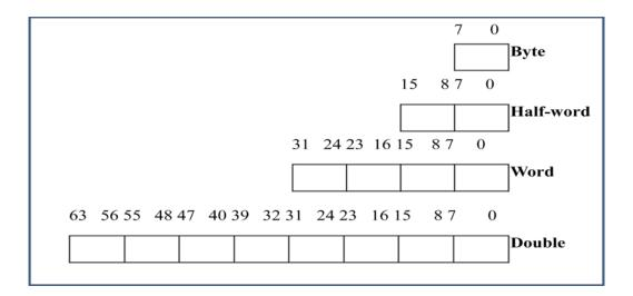
Figure 3: Fundamental Data Types
