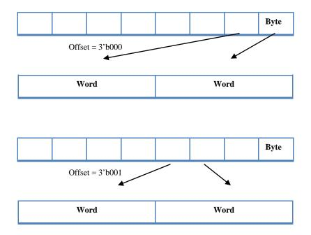
Figure 16: Type conversion- Rules for sign extension in the DATA LARs architecture
