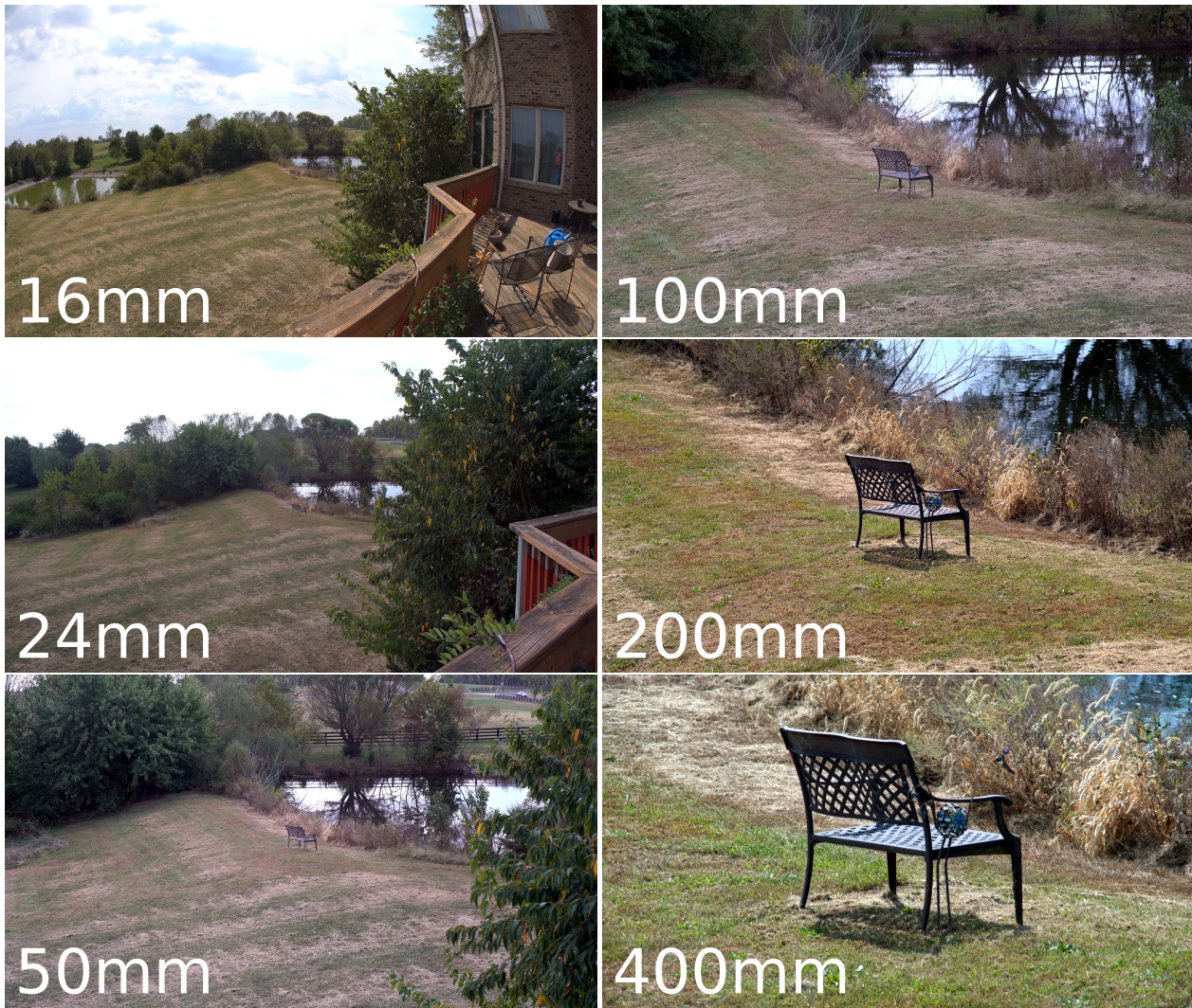
Figure 7. Sample images at 16, 24, 50, 100, 200, and 400mm; still-image motion blur is insufficient to estimate focal length except perhaps at 400mm
